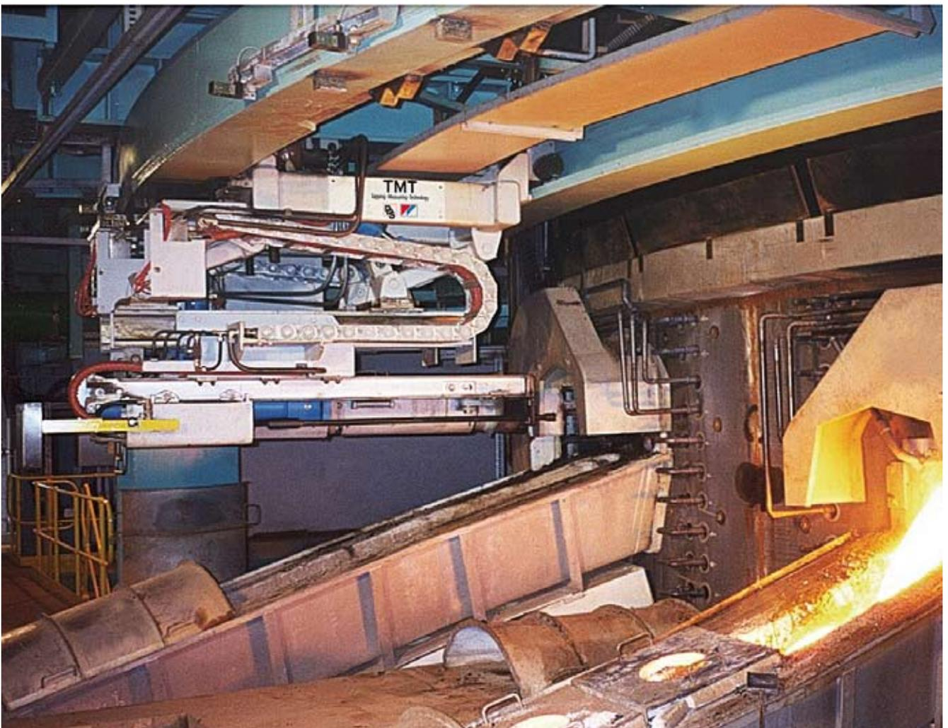
*Combined taphole machine after opening the furnace*
